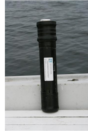
Oil detecting drifter buoy prototype developed in MSI, Taltech
