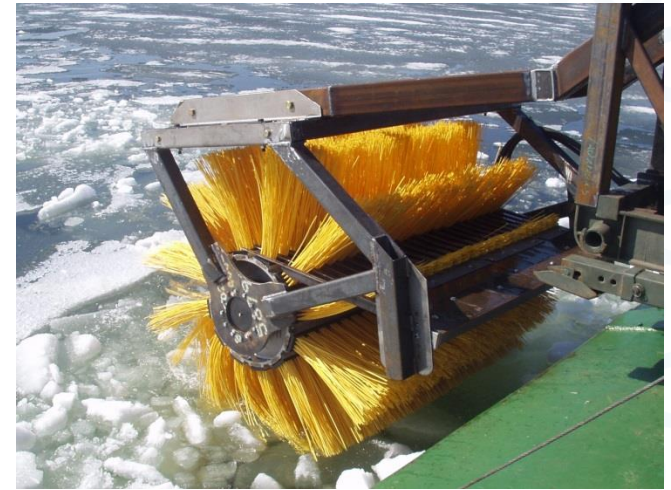
Oil recovery brush for ice conditions – prototype testing, photo SYKE
